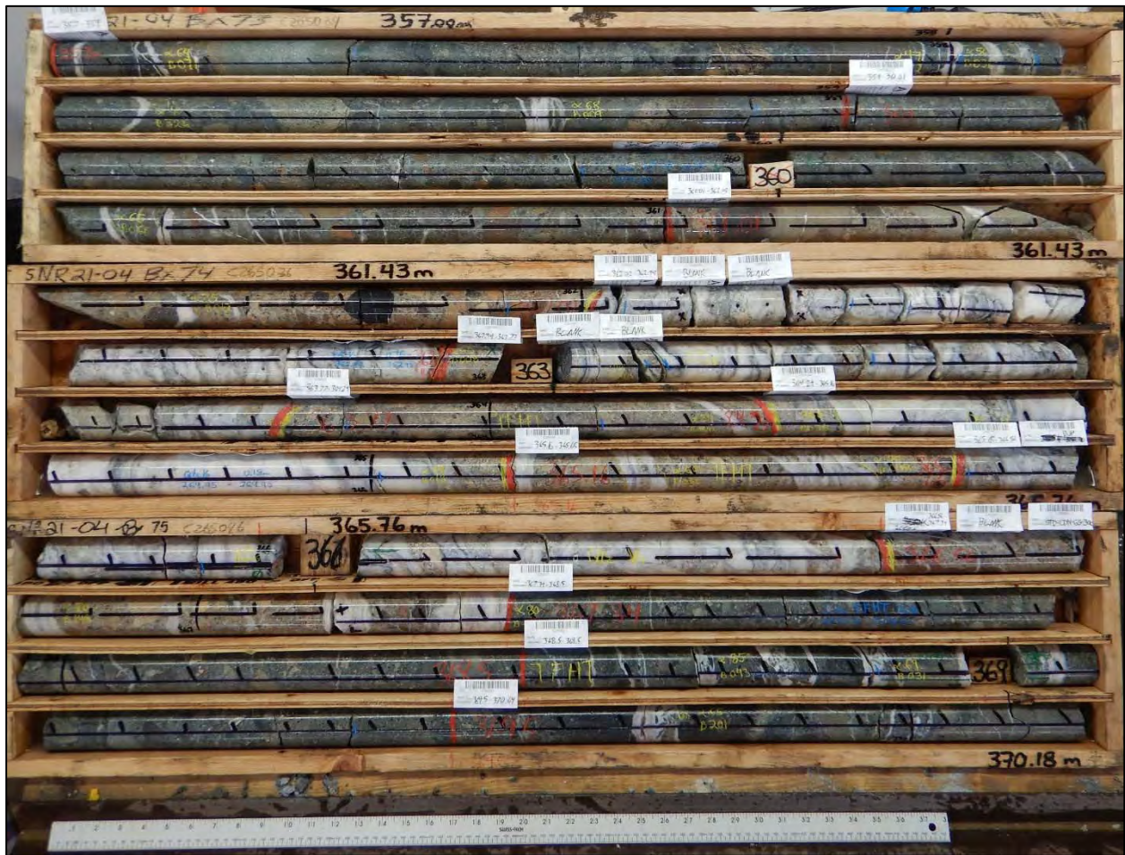
FIGURE 7.13 VEIN ZONE 3B IN DRILL HOLE SNR21-04 (357.00 M TO 370.18 M)
